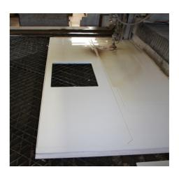
Do the entry hole outside respect the slab. In alternative make the hole a few centimeters from cutting perimeter and in any case, never less then 5mm. For inner holes, do always the input and output hole internally respect the part that you want to cut. Follow the below diagram (a low pressure for entry hole)
